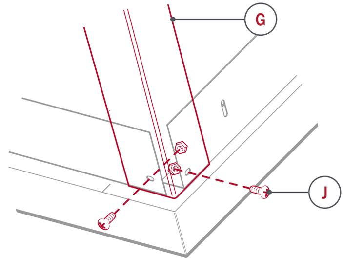
2. Use a straight head screwdriver to fasten 2 - Small screws and nuts (J). Place the screw head on the outside of the leg, and the nuts on the inside of the skirt.
