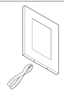
1. Cut the two (2) 1/8" plastic rivets located at the bottom of the door.
